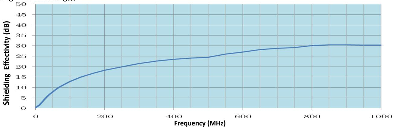
Test Condition 1.Film thickness : 25  $\mu$  m
